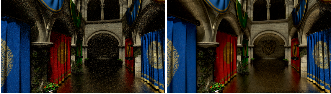
Figure 25: Difference between the default path tracer (left 106ms) and the reprojection method of 64 samples per step while reprojecting four samples per pixel (right 125ms). Both methods take four samples after the final rotation.
